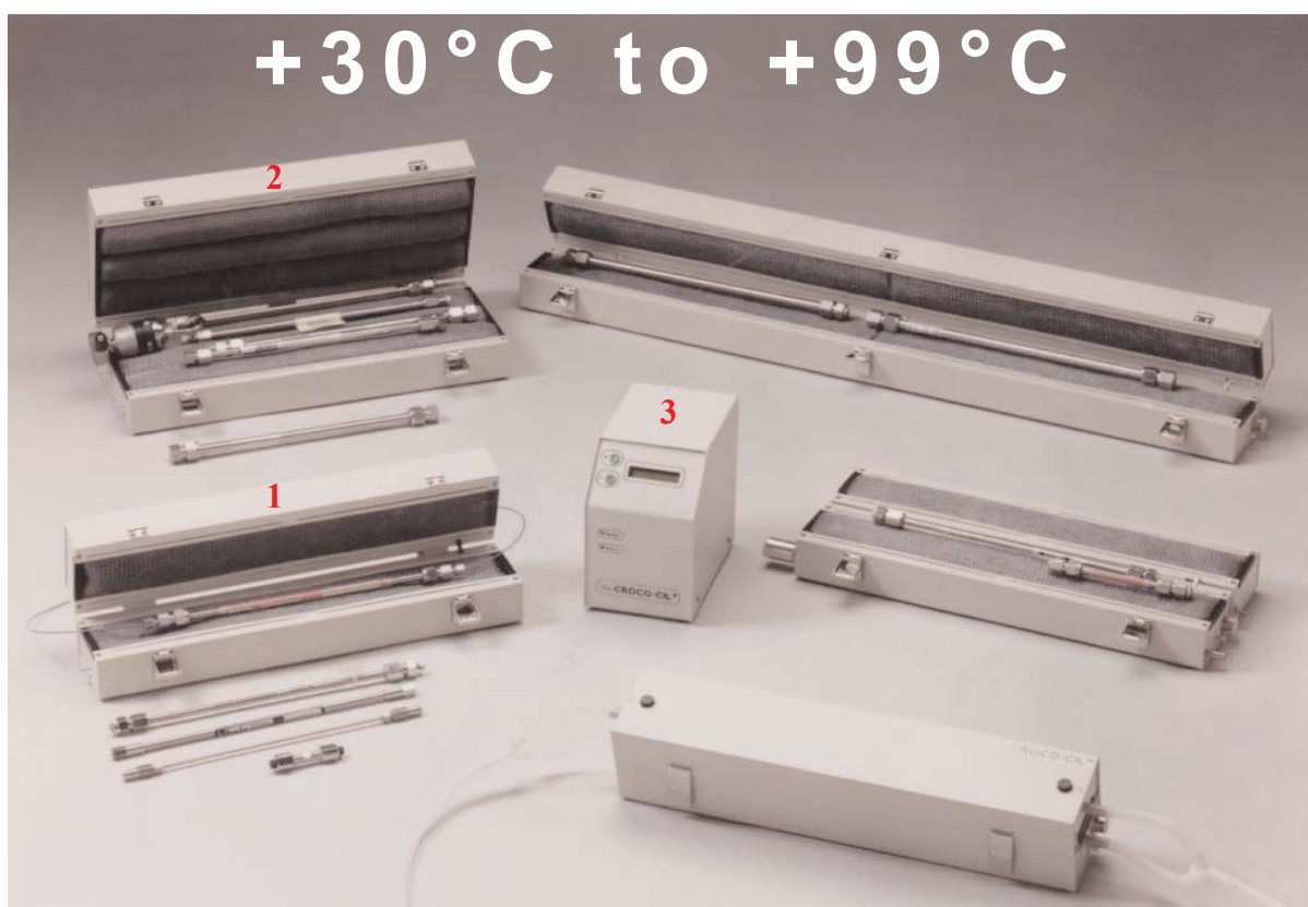
1 Oven 100 040 220P 2 Oven 100 040 220TW with Rheodyne Valve 7725i 3 Electronic regulator
